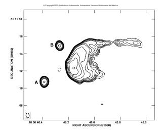
Fig. 1. VLA continuum contour map of G34.3+0.15 at 3.6 cm, made with natural weighting. Contour levels are -3, 3, 4, 5, 6, 8, 10, 15, 20, 40, 60, and 80 mJy/beam. The rms noise of this map is 0.46 mJy/beam. The ultra-compact components A and B are indicated. The half power contour of the beam, 0".55 × 0".37, with PA = 7°, is shown in the bottom left corner.
