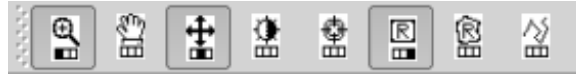
Figure 7.4: The ‘ Mouse Tool ’ Bar allows you to assign separate mouse buttons to tools you control with the mouse within the image display area. Initially, zooming, color adjustment, and rectangular regions are assigned to the left, middle and right mouse buttons, respectively.
